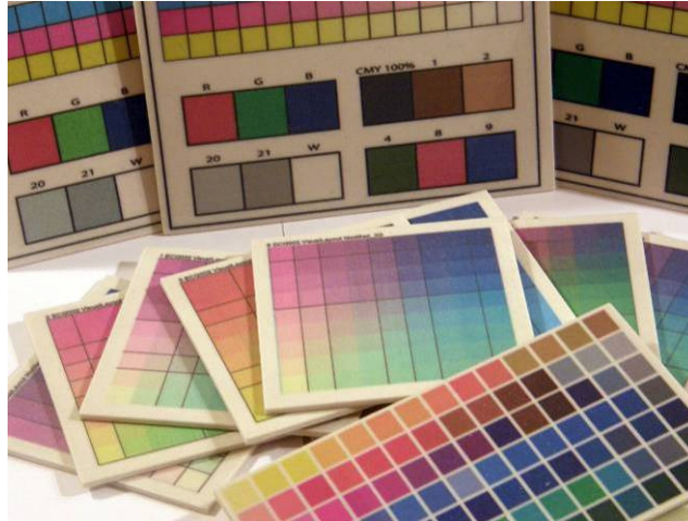
Figure 120. Example of custom designed and printed test colour charts in the form of plates
