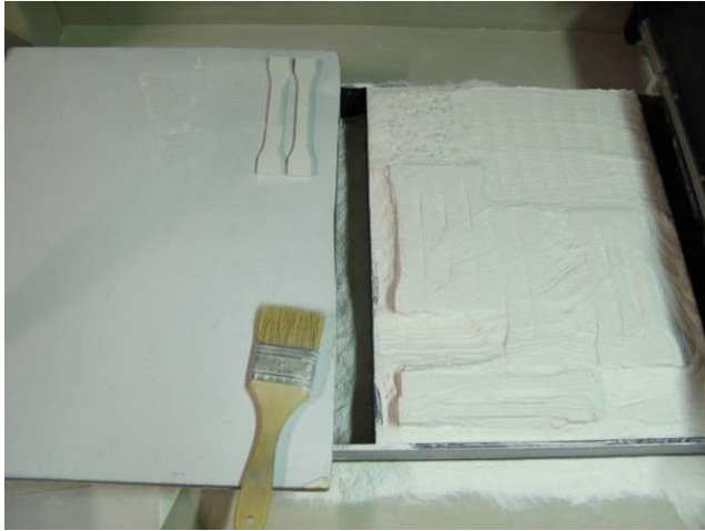
Figure 14. Post-processing, gross de-powdering, ZPrinter 510
