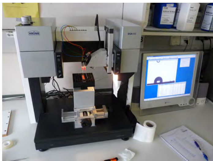
Figure 14: Krüß DSA 100 apparatus during measurement of RED sample.
