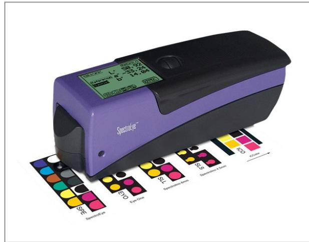
Figure 28. Spectrophotometer X-rite Spectroeye
