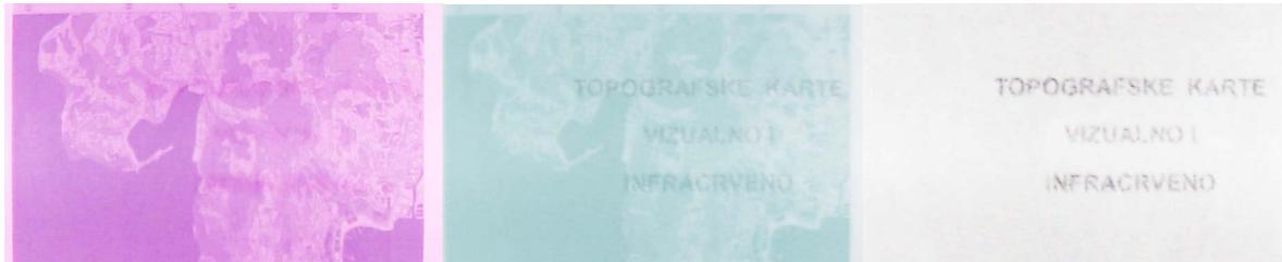
Figure 70. Scanned maps with barriers at: 570, 715 and 1000 nm
