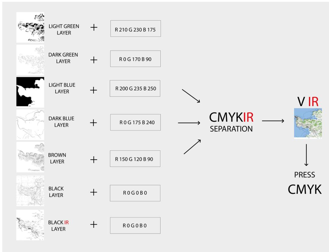
In CMYKIR, separation of black and white information comes from the layers, a color is assigned to each layer through their default RGB value and determines the color after printing. Constructed buildings and names of places are marked with Z (infrared) black dye, and V (visual) dye was used to mark roads and paths. Thus, the two highlighted colors in the same tone are completely isolated in the infrared spectrum.
