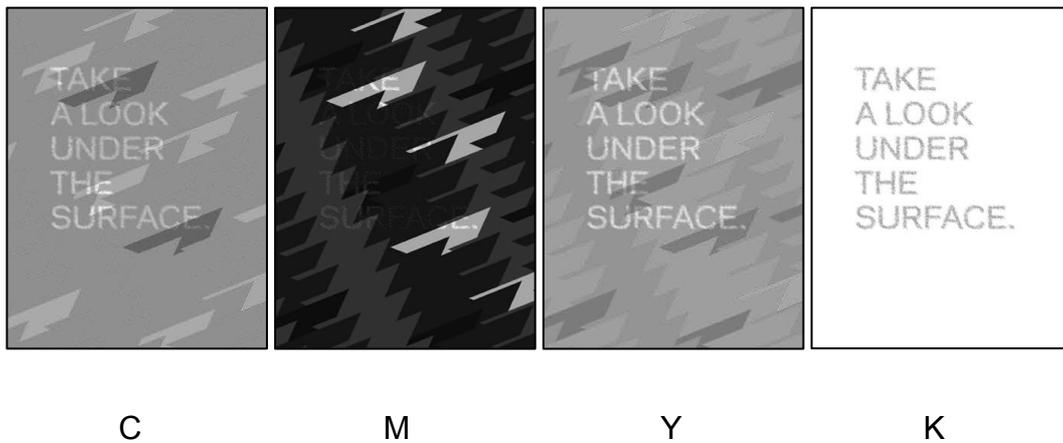
Figure 14. CMYKIR separation with planned image in K channel
